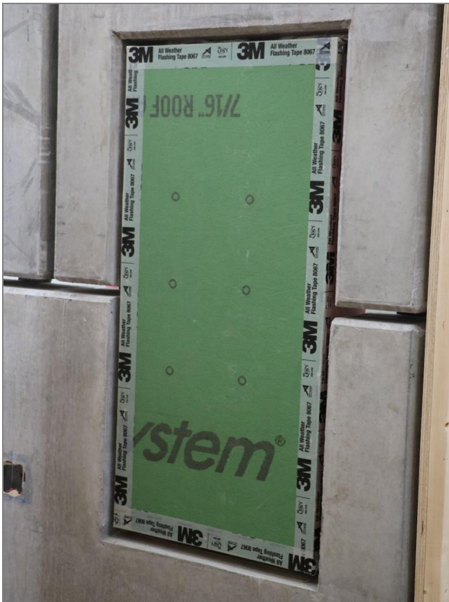
Figure 2.2 - Mock-up Wall 2, viewed from the outdoor side, showing surrogate window installed in rough-opening.
