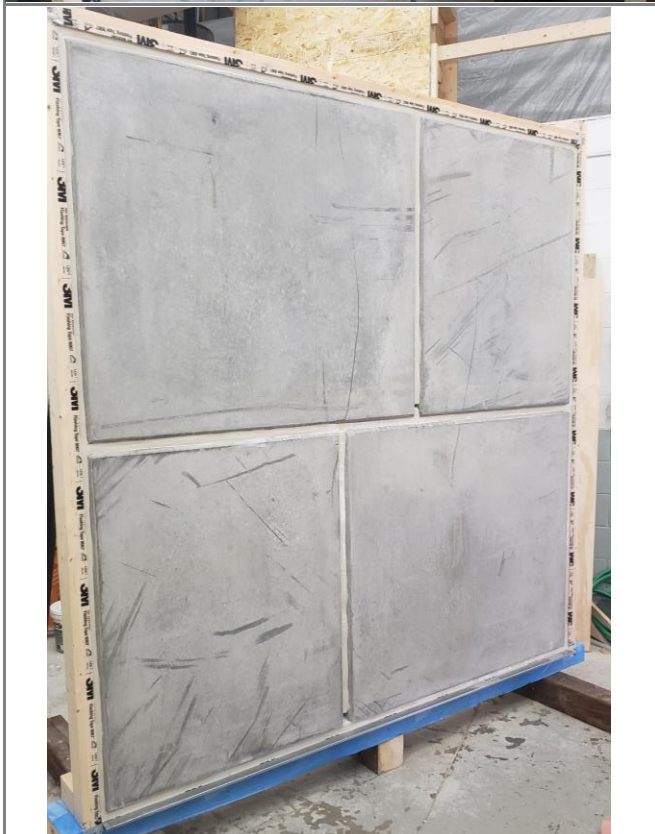
Figure 2.6 - Mock-up Wall 3 completed with perimeter frame and seals, ready for testing.
