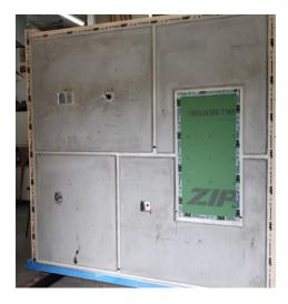
Figure 1 : Photographs of both the opaque and penetrated single wythe precast test wall specimens
